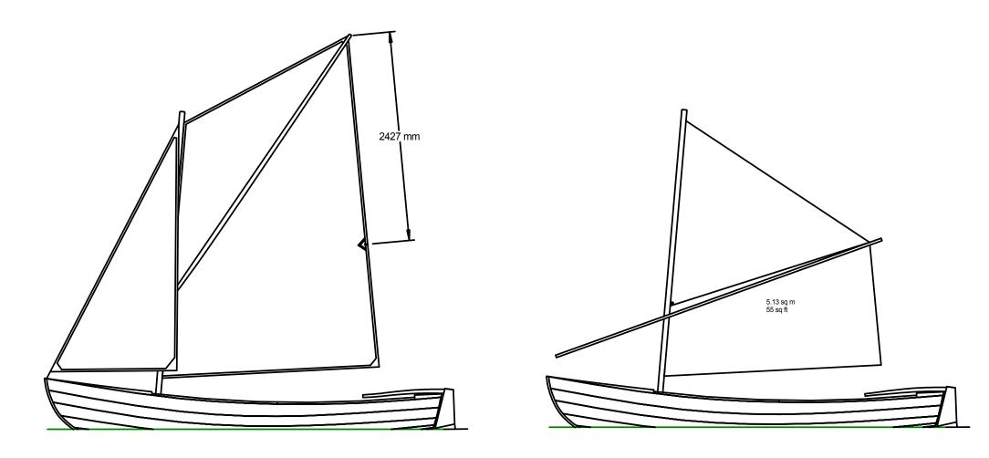
This drawing demonstrates the principle of "scandalizing" as a quick method of reefing. As you can see, the sprit is moved to a cringle on the leech positioned such that the head of the sail folds down neatly to be secured to the mast. This system can be used in addition (or as an alternative) to the conventional reefing shown on the sail-plan. Consult sailmaker.
